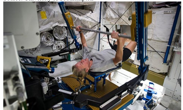
NASA astronaut using the Advanced Resistive Exercise Device (ARED) onboard the ISS. Credit NASA
